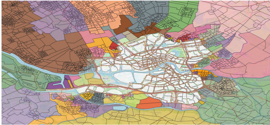
Figure 4.2: Zone layout for the external RODY zones (zoomed in on Rotterdam). White zones are the RODY zones in Rotterdam. All other colours represent a coupling to a VMRDH zone to an external link
