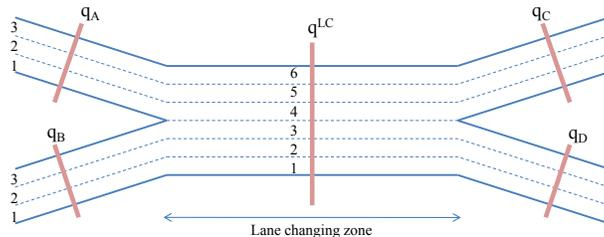
**FIGURE 9** Example of a weaving zone with detectors
