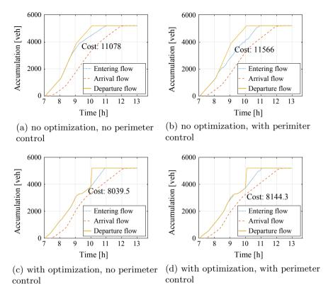
Fig. 73.3 Cumulative curves of departure, entering and arrival flow in four study cases. The cost in each case is put in each sub-figure
