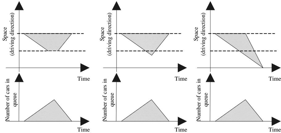
**Figure 1: Congestion dynamics in a space-time plane (upper figures) and number of cars in a queue (lower figure). From left to right: implementation of a) a vertical queuing model, b) horizontal queuing model, c) shockwave theory**
