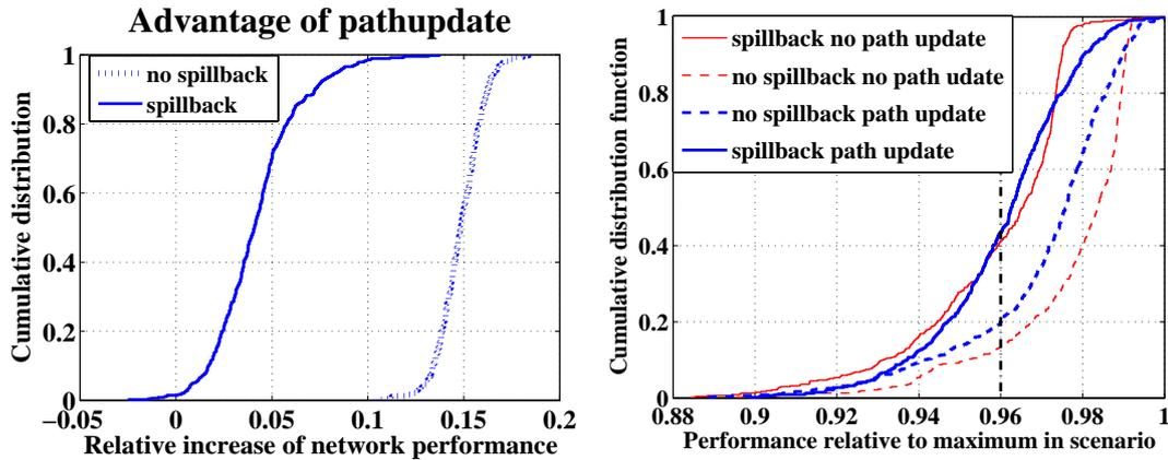
**Figure 2:** a) Cumulative distribution function of the advantage of the network performance when applying path updates; b) the cumulative chances that the network performance decreases more than a certain level (horizontal axis) if a randomly chosen link is blocked.
