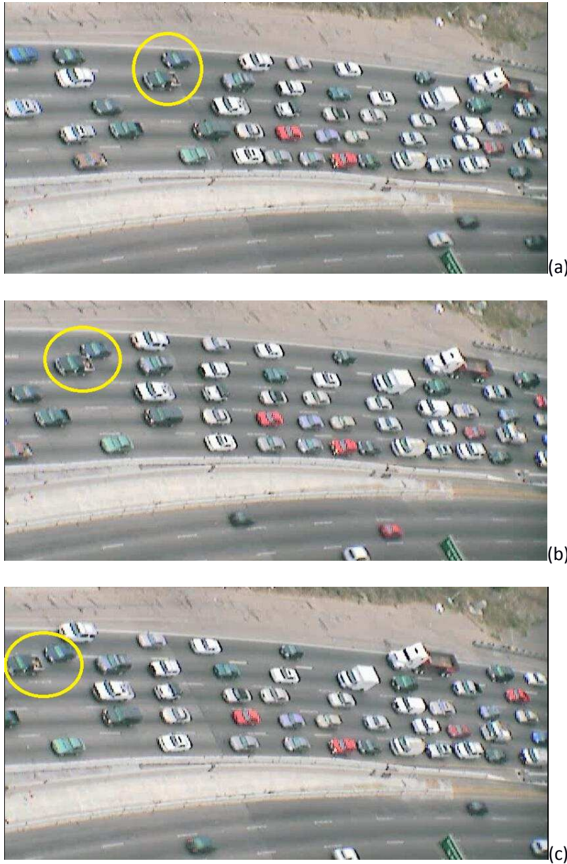
Fig.8. The special lane changes found at camera 8: the front gap in the target lane is smaller than 0. (a) 0:19; (b) 0:21; (c) 0:23.
