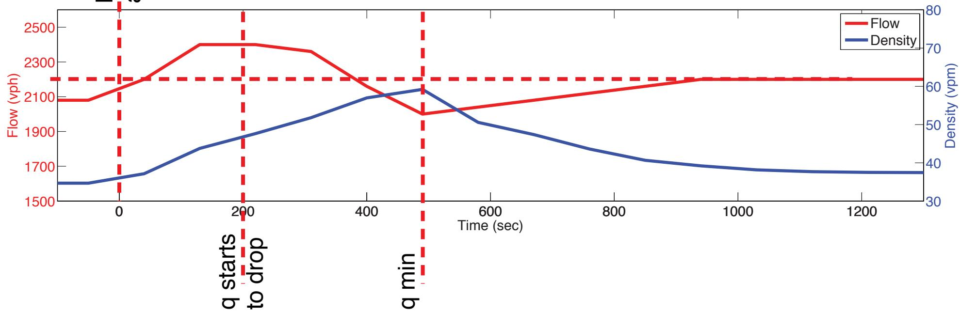
An empirical study would see  $q$  drop around 200 sec, take the highest throughput prior to that point and (erroneously) call it capacity
